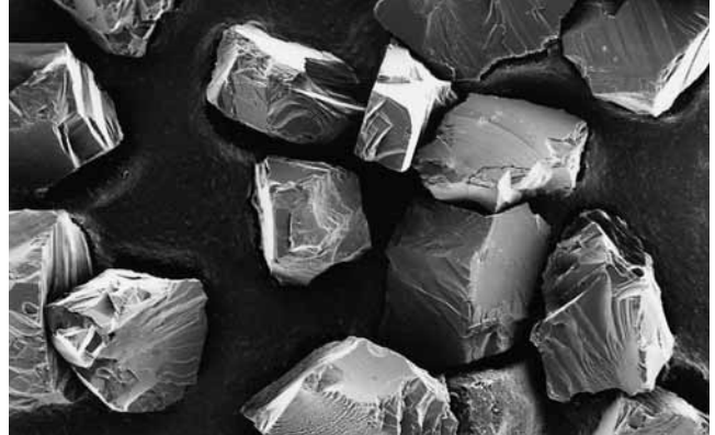
Sharp edges of monocrystalline diamonds of MetaDi ® Diamond Paste ensure clean and efficient cutting action.
