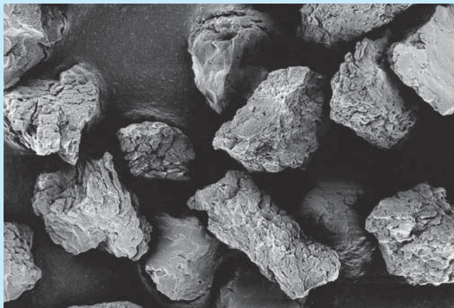
Angular, blocky-shaped polycrystalline diamonds of MetaDi ® Supreme provide numerous cutting facets on the particle surface, resulting in less deformation.
