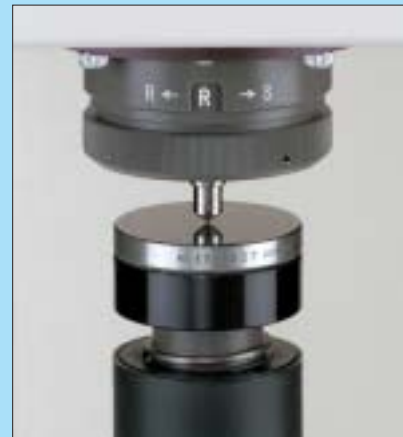
Simple change over between Rockwell and Rockwell superficial pre-load application for the twin model.
