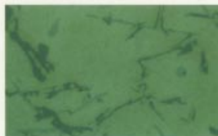
Aluminum silicon alloy prepared with MASTERMET 2 Colloidal Silica Suspension. Brightfield - 400x.
